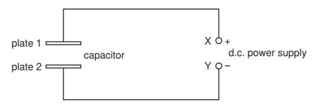
Along which paths do electrons flow as the capacitor starts to charge?
